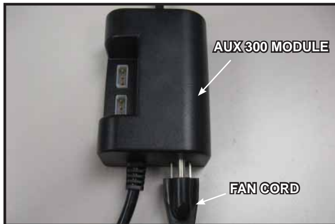
Figure 6. Plug Fan into AUX300 Module
